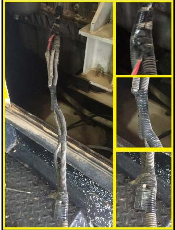
STEP 4. Replace any damaged sections of the ¾" corrugated wire loom from the DC alternator going past the fuel filter assemblies. Wrap electrical tape around the harness and connectors temporarily in order to form a narrow profile to ease the installation of the heat sleeve material.
