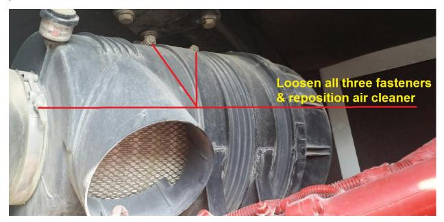
**Step 2.** With the air cleaner repositioned simply retighten the three fastener bolts. Please refer to the illustration below for the finished view.
