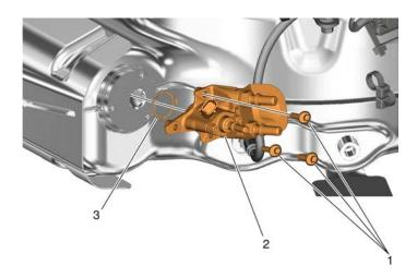
Remove and discard the aftertreatment DEF dosing valve fasteners. Remove the aftertreatment DEF dosing valve from the aftertreatment diesel particulate filter (DPF) and place in a suitable graduated collection container. Discard the DEF dosing valve gasket.
