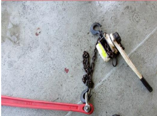
Figure 1 – Pipe wrench used with Come-a-long and Shackle
