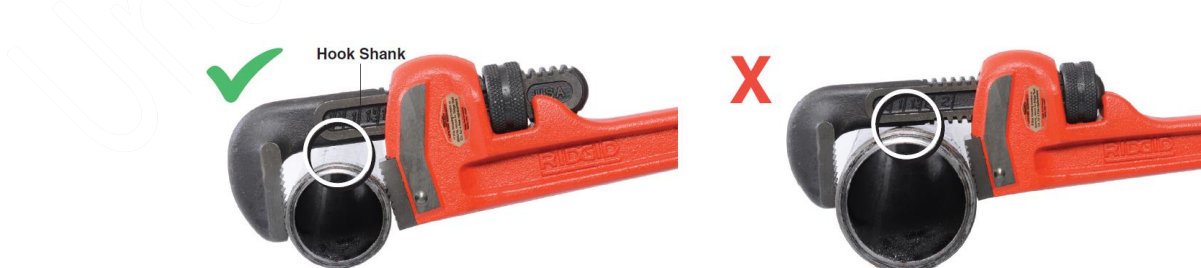
Figure 2 – Proper loading of Pipe Wrench
