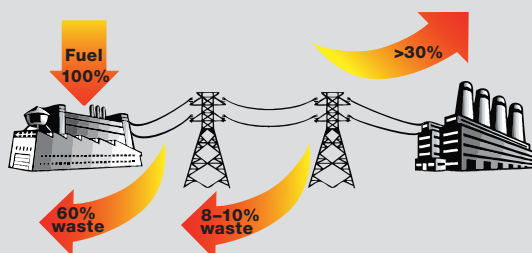
Figure 1 - Today's "grid" system of central power plants and transmission lines wastes much of the energy in the original fuel.
