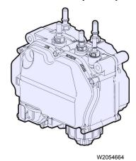
This information provides the correct procedure for replacing the diesel exhaust fluid (DEF) filter in the DEF pump on MACK US2010 emissions compliant vehicles.
