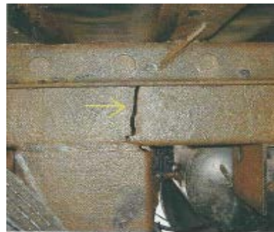
Cracked Trailer Frame Member
