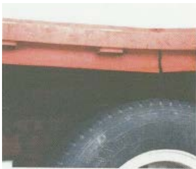
Cracked Trailer Frame Member Frame Member
