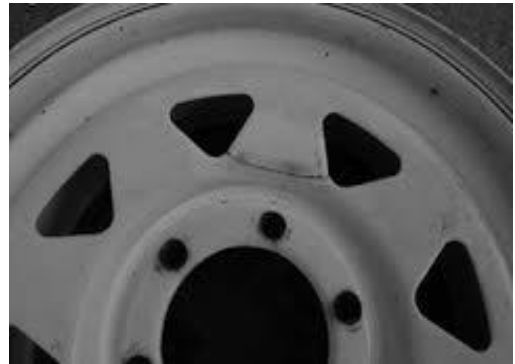
Cracked Wheel/Hand Holds
