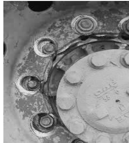
Missing Nuts/Broken Studs
